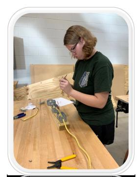
completed their electrical board projects. Students learned about electric and electric wiring and were then asked to create and wire a board with a switch, light, and receptacle on it.
